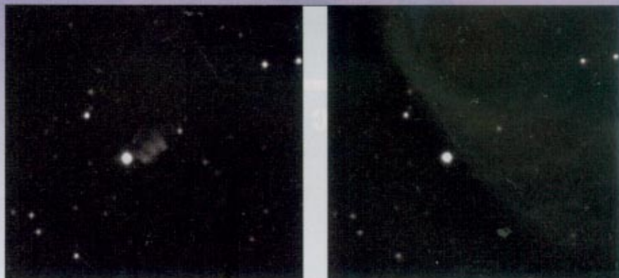
Figure 1. Astronomical exposures showing a normal star field (right) and the same star field with RBI (left).
