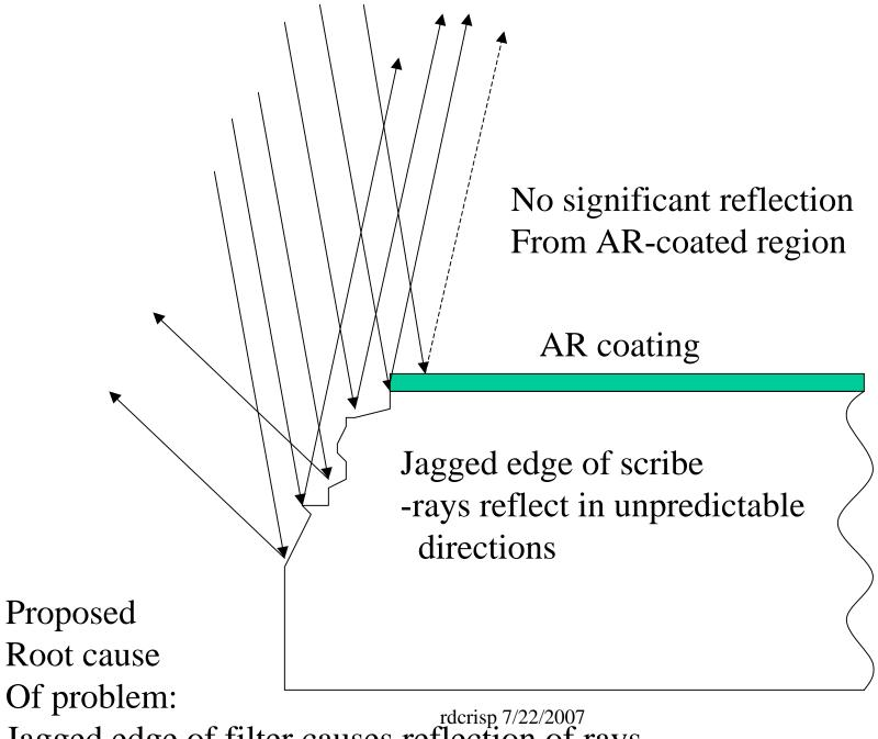
Jagged edge of filter causes reflection of rays
