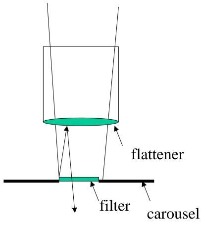
Theorized cause: reflection of passband signal from Filter edge
