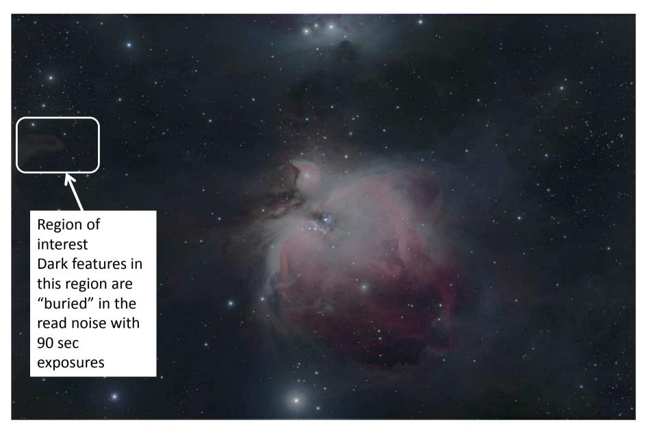
ABG Sensor (KAI29050) with 20,500 e- saturation signal on HDR object (M42)
